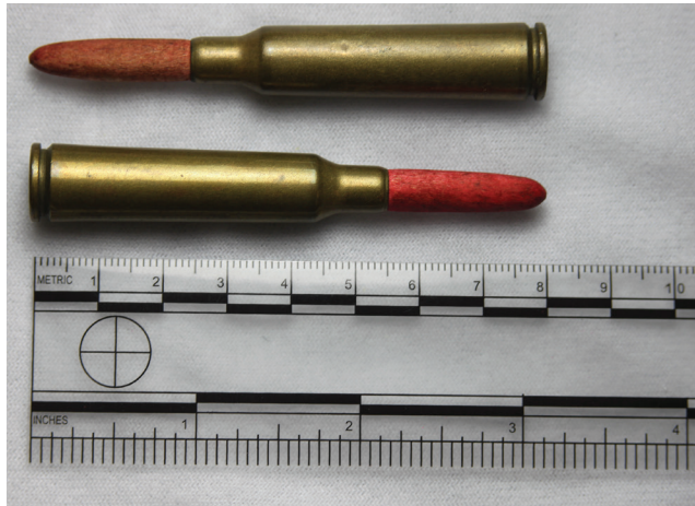
Figure 2.37 Swedish 6.5mm cartridges loaded with wooden projectiles. (Image from author's collection.)
